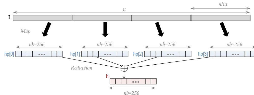
Figure 2. Safe parallel implementation of histogram computation.  $nt = 4$
